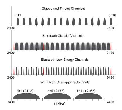
Wireless coexistence technologies allow multiple technologies, including Wi-Fi, Thread, Zigbee, and Bluetooth LE, to operate on the 2.4GHz band without signals from one radio interfering with adjacent radios. Several alternatives exist to implement Wi-Fi coexistence on gateways and they are generally divided into **unmanaged** and **managed** techniques.
