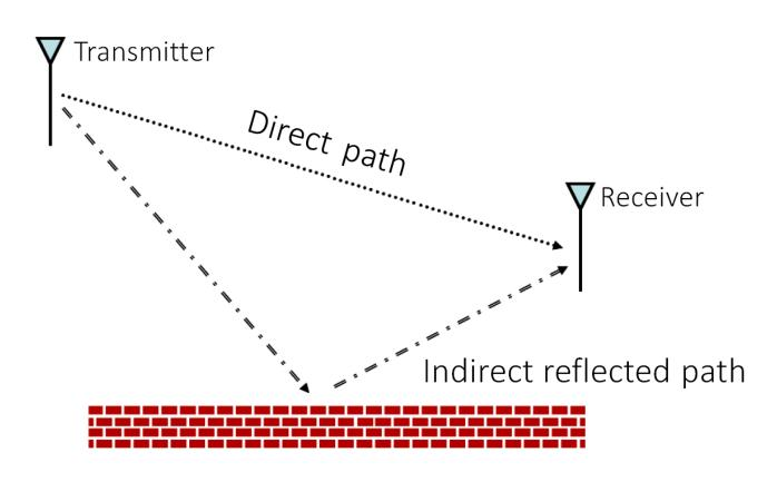
Multipath propagation: Line of sight (LOS) signal path vs. reflected signal
